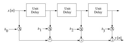
where  $b_0 = 1$ ,  $b_1 = 0$ ,  $b_2 = \frac{1}{2}$ ,  $b_3 = \frac{1}{2}$ , determine its impulse response h[n].
