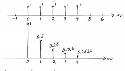
(c) For a four point running averager, the impulse responde is  $A[n] = \frac{1}{4} \left( \delta[n] + \delta[n-1] + \delta[n-2] + \delta[n-3] \right)$
