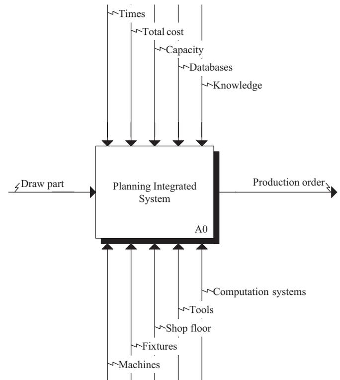
Fig. 2. Initial level of the IDEF model.
