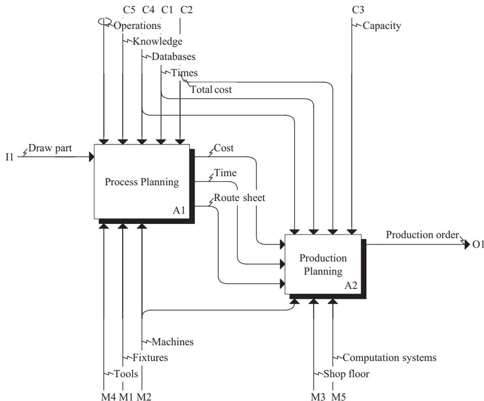
Fig. 3. First level of the IDEF model.
