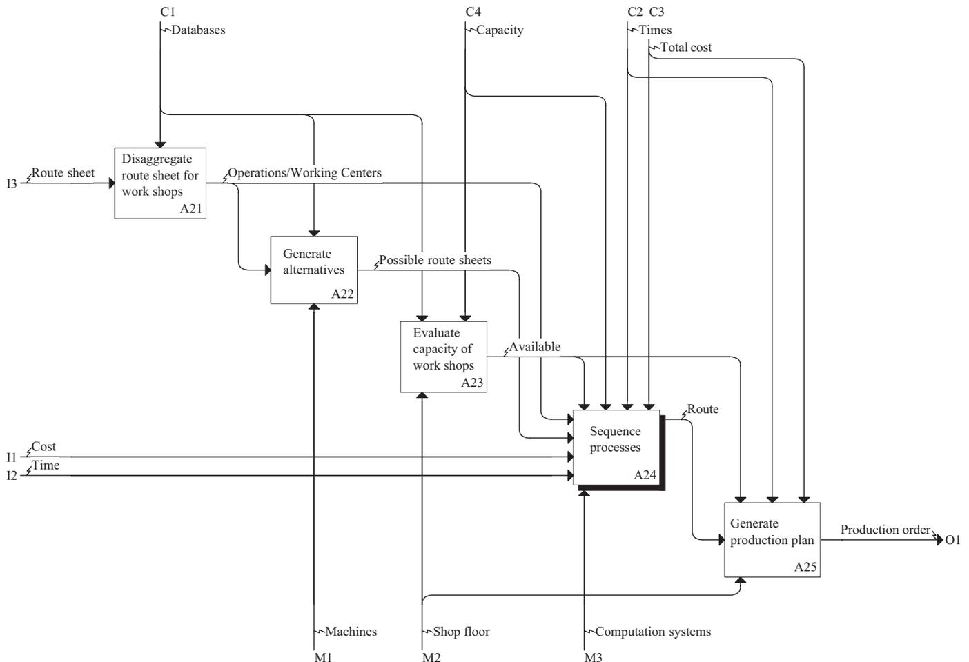
Fig. 5. Production planning level in the IDEF model.
