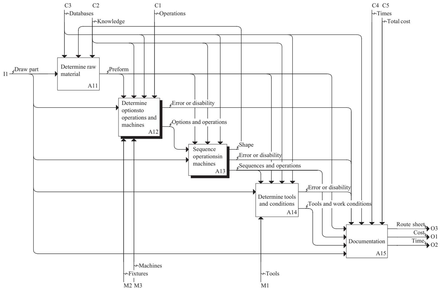
Fig. 4. Process planning level in the IDEF model.
