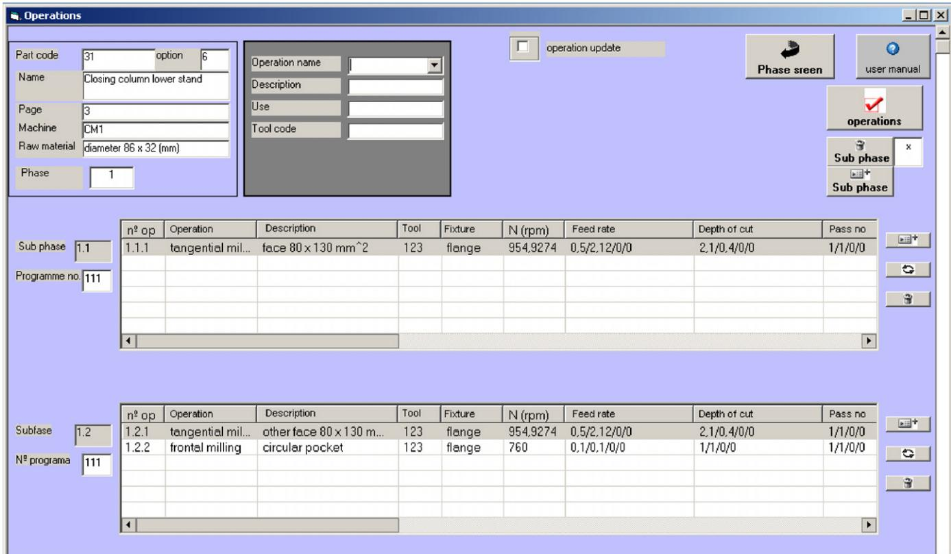
Fig. 8. Operations screen with one input operation for sub-phase 1.1 and two operations for sub-phase 1.2.
