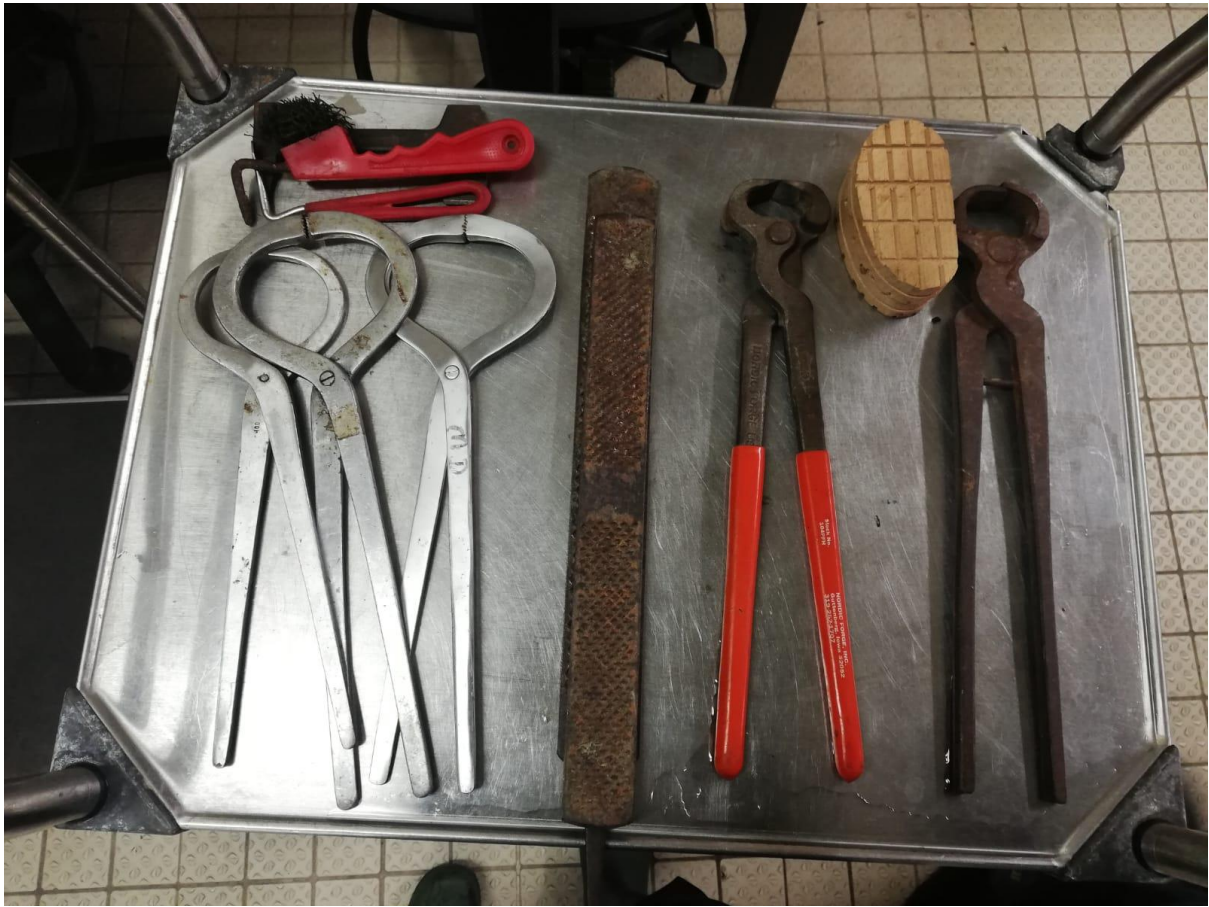
SHOWN IN PICTURE: HOOF TESTERS (L), RASP (M), HOOF BLOCK (TOP R), HOOF PICK WITH BRUSH (TOP L), HOOF NIPPERS (R)
