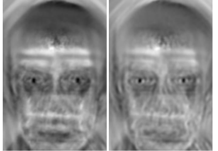
Fig. 7. The output of the correlation with an SDF computed using the spectral envelope of 20 training images as whitening preprocessing. Left: the normal SDF (20 examples). Right: a least square SDF with 6 templates (20 examples). The darker the image the higher the corresponding value. The least square SDF exhibits a sharper response using the same whitening filter.
