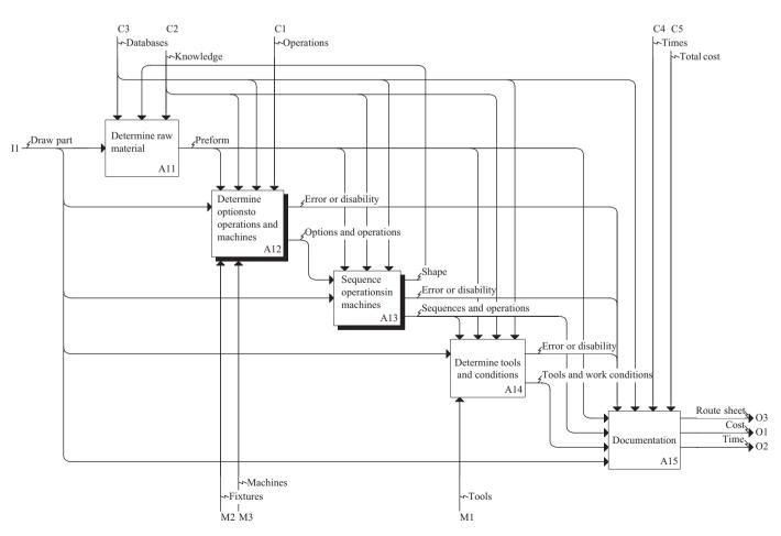
Fig. 4. Process planning level in the IDEF model.
