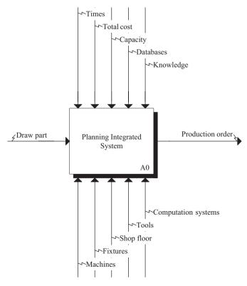
Fig. 2. Initial level of the IDEF model.
