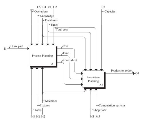
Fig. 3. First level of the IDEF model.
