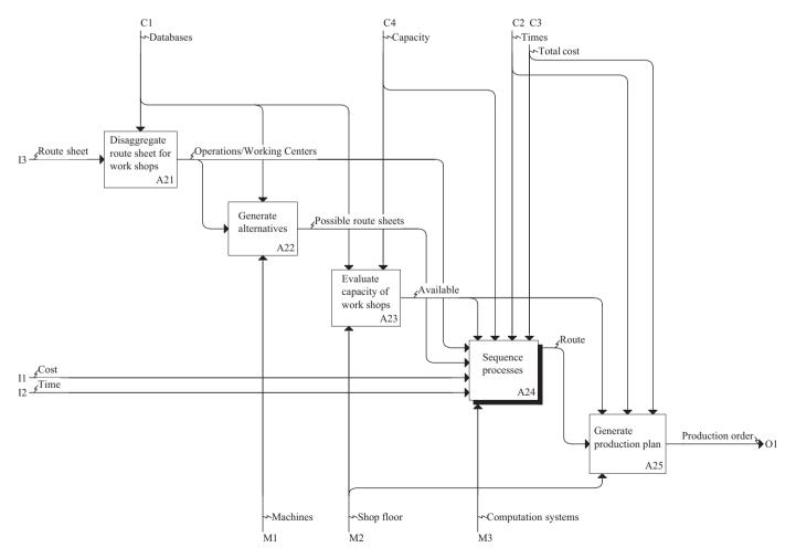
Fig. 5. Production planning level in the IDEF model.
