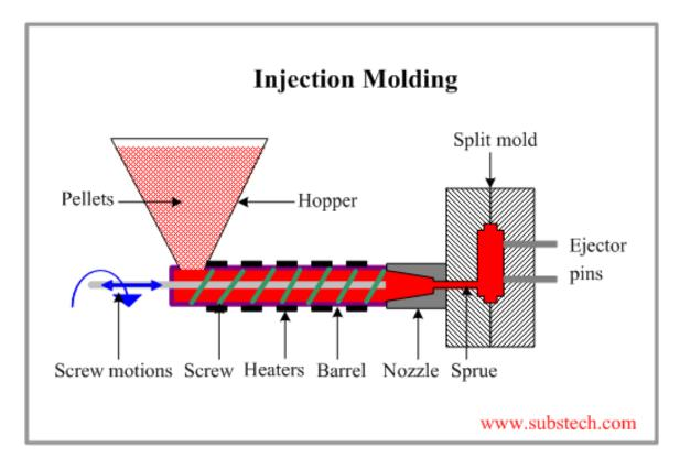
Injection molding is where you have a cast with an entry spout, and you pour the material into the cast (much like with slip casting) only you leave all the material in the mold to cool/dry/harden, and then you have a solid mold of your object.
