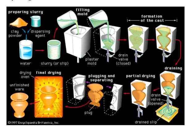
Slip casting is when you have a mold of the object that you want to create, and you pour a very thin clay material (slip) into the mold. You leave it there long enough to coat the mold, then pour out the excess. As the inside of the mold dries, you get a shell of the object you're molding. When fired, it becomes the final molded object.
