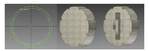
Next is to figure out how to make this so it would mate to a lid that would fit over it a twist. I think I am going to cut the outer portion down about 15mm, leaving a circular protrusion in the middle. This should have an added bonus of making the watch sit more center mass if you will. I am going to need some sort of a stop for the lid to hit when it is lined up, and a lip to hold it on.
