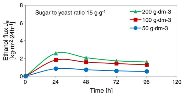
Fig. 7. Changes in ethanol flux as a function of time during the fermentation in a MDBR. Feed temperature: 310 K.
