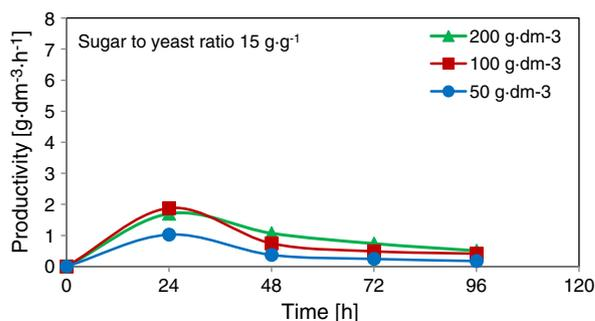
Fig. 10. Changes in productivity in time during the fermentation in a classical reactor. Feed temperature: 310 K.
