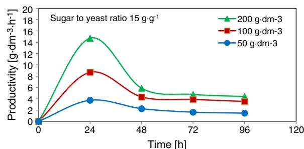
Fig. 9. Changes in productivity in time during the fermentation in a MDBR. Feed temperature: 310 K.
