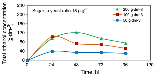
Fig. 8. Changes in total ethanol concentration as a function of time during the fermentation in a MDBR. Feed temperature: 310 K.
