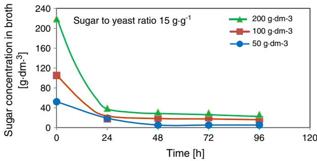
Fig. 3. Changes in sugar concentration in the broth as a function of time during the fermentation in a MDBR. Feed temperature: 310 K.
