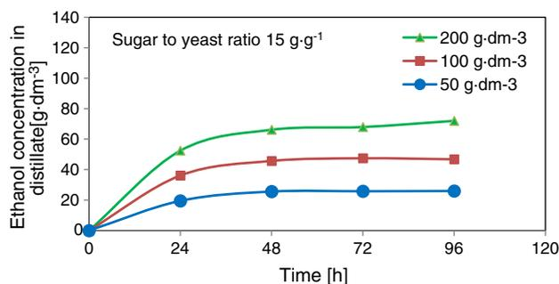
Fig. 6. Changes in ethanol concentration in the distillate as a function of time during the fermentation in a MDBR. Feed temperature: 310 K.
