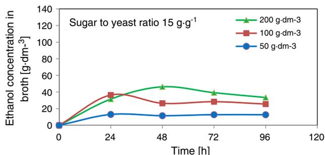
Fig. 2. Changes in ethanol concentration in the broth as a function of time during the fermentation in a MDBR. Feed temperature: 310 K.
