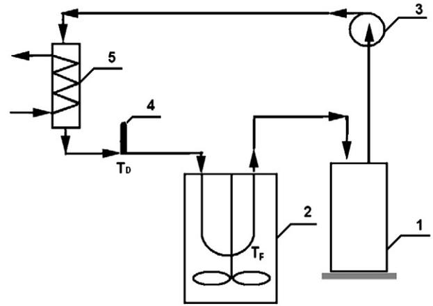
Fig. 1. Scheme of the experimental apparatus. 1— distillate tank, 2— bioreactor with capillary module, 3— pump, 4— thermometer ( $T_D$ —temperature of the distillate), 5— cooling system.
