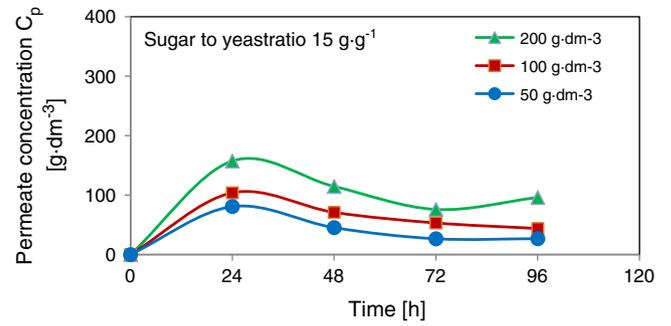
Fig. 5. Changes in ethanol concentration in the permeate as a function of time during the fermentation in a MDBR. Feed temperature: 310 K.
