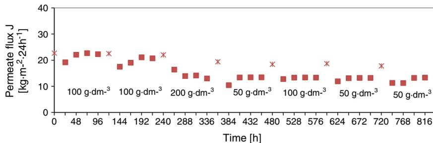
Fig. 4. Changes in permeate flux as a function of time during the fermentation in a MDBR. Feed temperature: 310 K. \*permeate flux for distilled water used as a feed performed after the fermentation in the MDBR.
