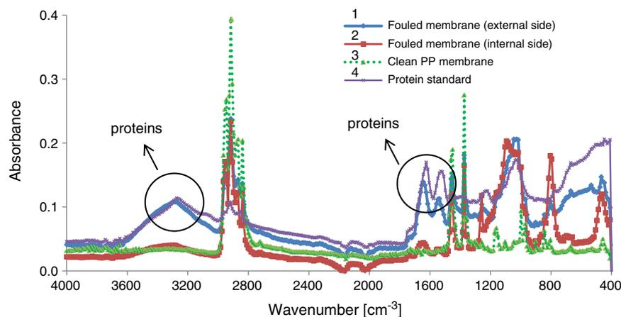
Fig. 11. FT-IR spectra of clean polypropylene membrane, fouled membrane after the fermentation in a MDBR and dry protein standard.
