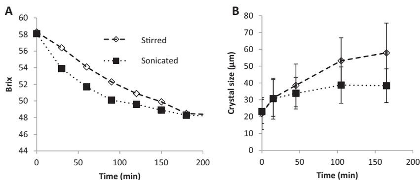
**Fig. 3.** Change in Brix (A) and crystal size (B) at a flow rate of 11 L/min. Sonication was applied at an energy density of 3.3 J/mL.
