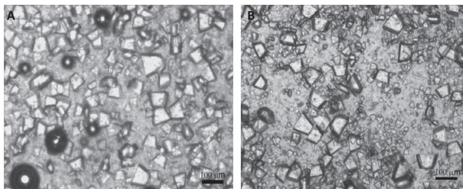
Fig. 5. Crystal morphology and distribution viewed under a light microscope at 10× magnification following stirring (A) and sonication (B).
