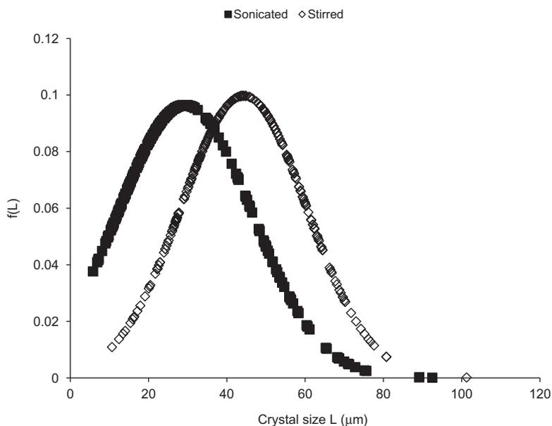
Fig. 4. Normalised crystal size distribution of stirred and sonicated whey at the end of crystallisation.
