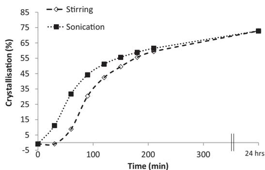
Fig. 6. Crystallisation of stirred and sonicated whey; sonication was delivered at a flow rate of 1 L/min and an applied energy density of 15 J/mL.
