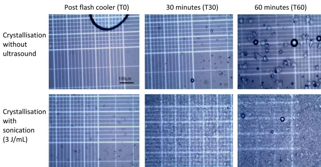
**Fig. 2.** Concentrated whey viewed under a light microscope at 10 $\times$  magnification immediately after flash cooling at a flow rate of 2 L/min and after 60 min (scale bar applies to all images).
