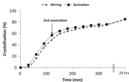
Fig. 7. Crystallisation of stirred and sonicated whey; initial sonication was delivered at a flow rate of 11 L/min and an applied energy density of 6 J/mL. A second treatment of ultrasound was delivered during crystallisation at 120 min and an applied energy density of 4 J/mL.
