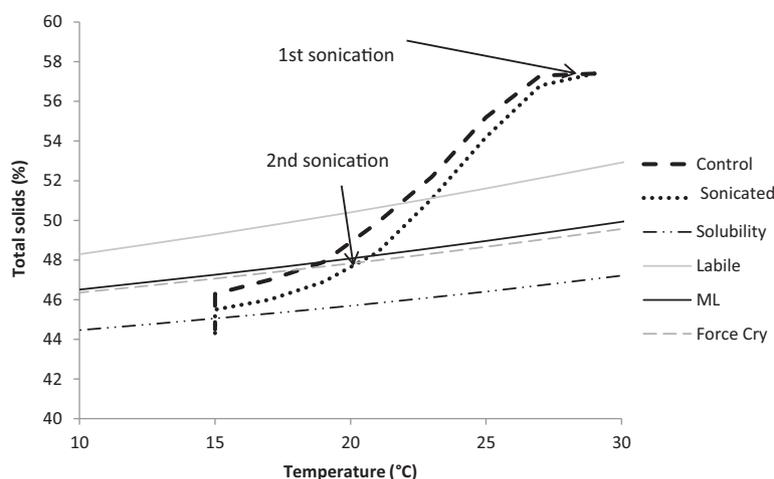
**Fig. 8.** Crystallisation profile of stirred and sonicated whey showing lactose solubility, forced crystallisation and the labile and metastable zones. Initial sonication was delivered at a flow rate of 11 L/min and an applied energy density of 6 J/mL. The second batch treatment of ultrasound was delivered at an applied energy density of 4 J/mL.
