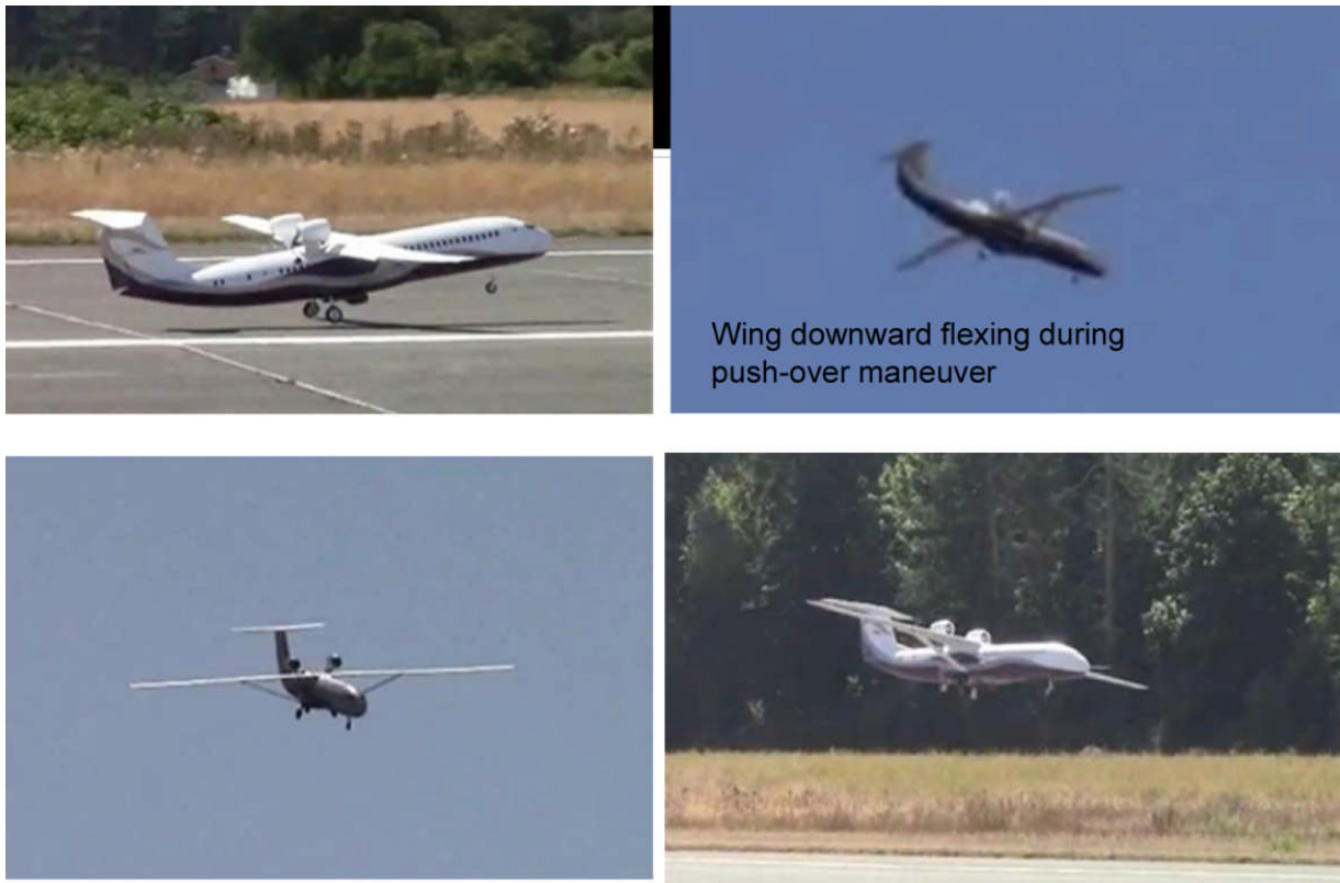
Figure 49: The 2011 University of Washington SBW UAV in flight, Summer 2011.
