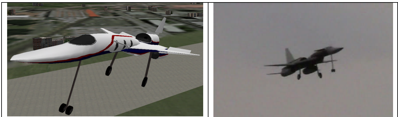
Figure 7: An X-Plane simulation model of the 2006 UAV and the actual UAV in flight.
