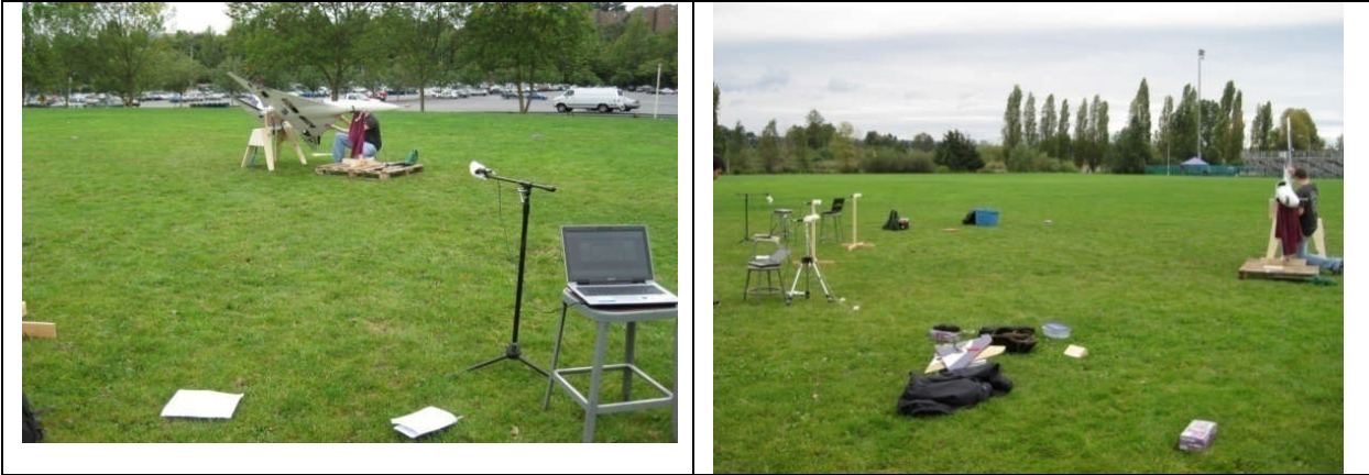
Figure 39: Noise testing over grass 360 degrees around the 2010 UAV at different bank angles.
