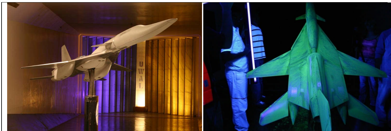
Figure 3: A 2006 model of a supersonic cruise configuration installed at the University of Washington's 12' x 8' low speed Kirsten Wind Tunnel (left) with China Clay flow visualization patterns at a high angle of attack (right).
