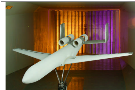
Figure 16: The 2008 UAV: the wind tunnel model in the Kirsten wind tunnel (left) and the NASTRAN model (right) showing mesh details and non-structural masses.
