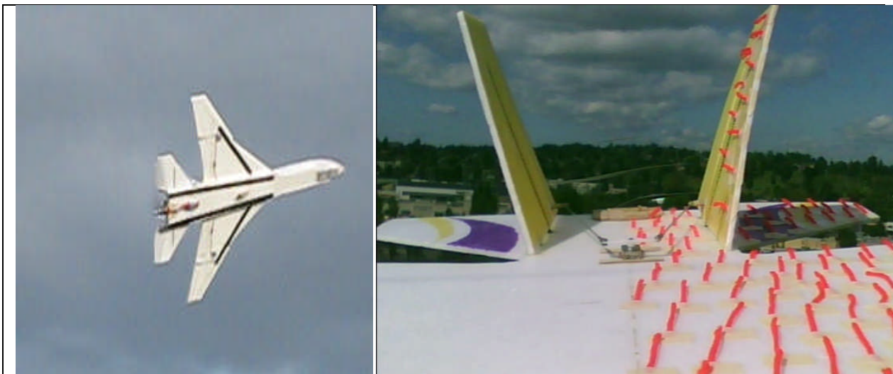
Figure 37: The “2010 “foamie” – a ½ scale avionics systems testbed for the 2010 UAV. On the right – tufts used to study the flow field over the wing during maneuvering flight.
