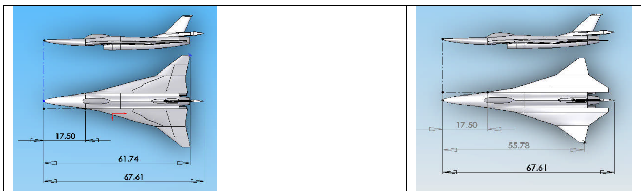
Figure 9: The two finalist competing design for the modification of an F16-XL to a low-boom research aircraft.
