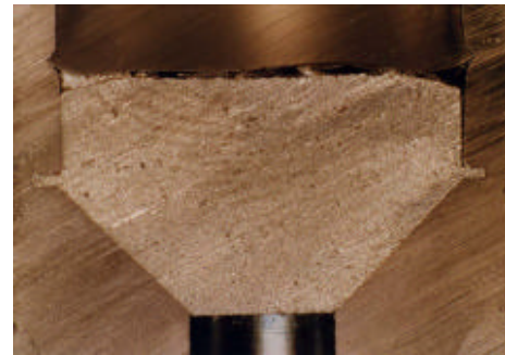
Fig. 17 Cut section of the freeze seal after 2000 hours operation ( RAPID )
