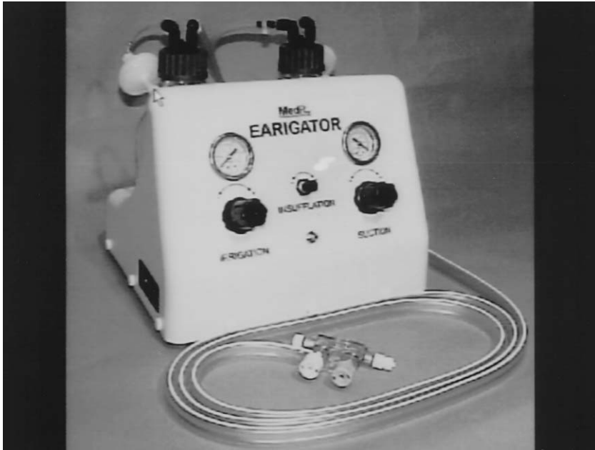
Fig. 1. The Earigator. This flush and suction unit provides adjustable flushing volumes adequate for irrigating the tympanic bulla. Trumpet valves in the handpiece allow flushing and suctioning with one hand.
