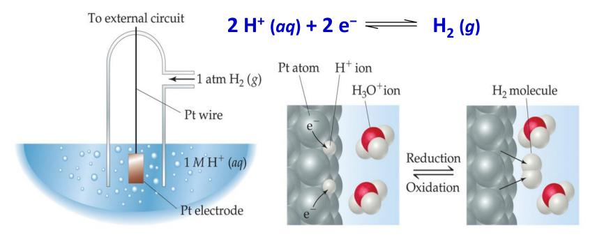
The platinum electrode has a large surface area so that it can establish an equilibrium between  $H_2(g)$  and  $H^+$  (aq) as rapidly as possible.
