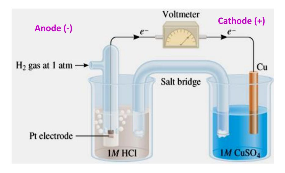
SHE is anode and Cu<sup>2+</sup>(aq)/Cu(s) half-cell is cathode.
