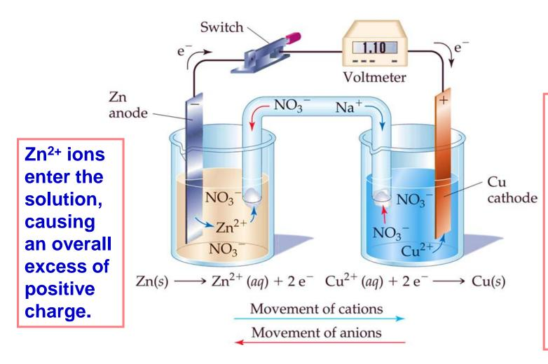
Cu<sup>2+</sup> ions leave the solution, positive charge removed, leaving excess of negative charge.
