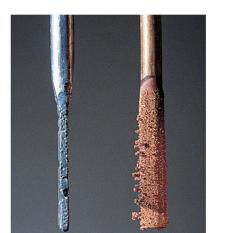
Cu is deposited at Cu electrode
