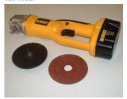
**Dewalt Cordless Cutoff Tool** (Angle Grinder) Above, with battery pack attached, along with a Dewalt Backer Pad (left), and an aluminum oxide 24 grit abrasive pad (right). This tool performs many of the tasks of a conventional rasp.
