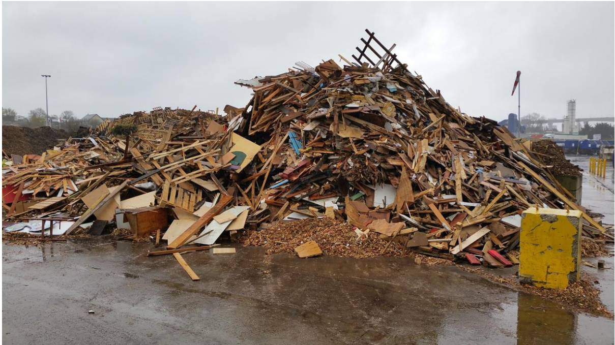
A pile of Class B waste wood [Wood products that may contain glue, finishes (paints, varnishes, stains, etc.), metals (nails, screws) and plastics].
